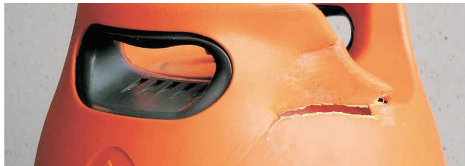
Figure 2b Impact Damage (level 2) - Repairable
