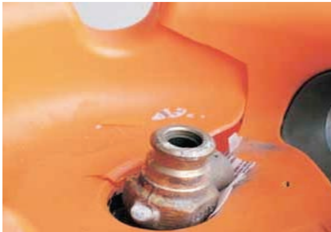
Figure 4 Structural damage (level 3) - Not Repairable
