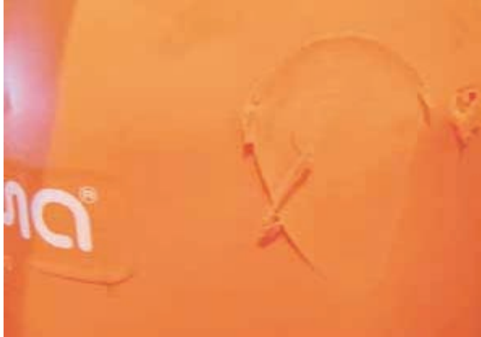
Figure 3a Superficial Heat Damage (level 2) - Repairable
