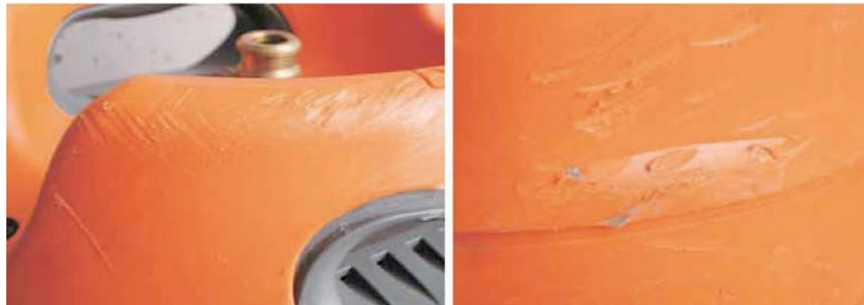
Figure 1a Abrasion Damage (level 1) – Serviceable
