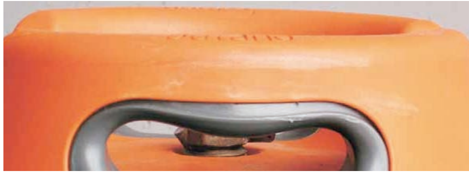
Figure 2a Impact Damage (level 1) - Serviceable
