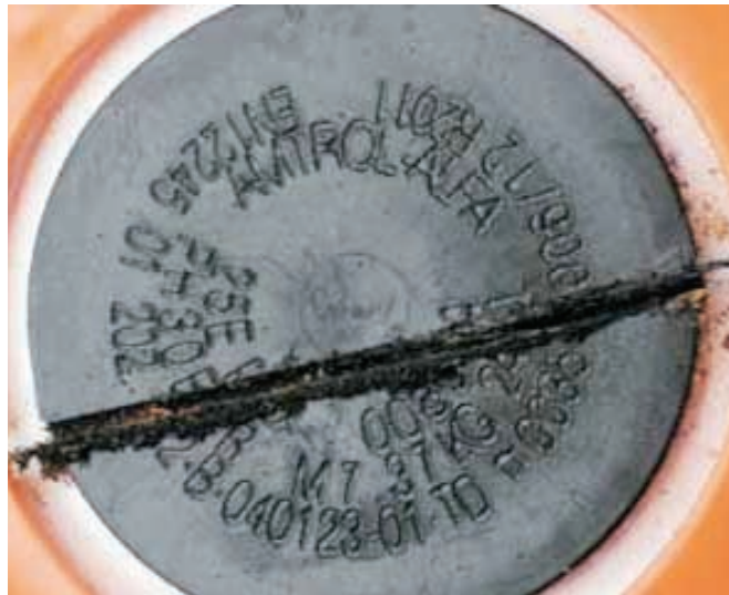
Figure 6 Marking Illegible (level 2) - Repairable
