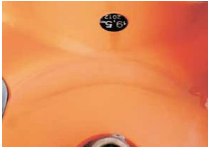
Figure 5 (24 hours after attack damage with H 2 SO 4 - 98%) Chemical Attack Damage (level 2) - Repairable
