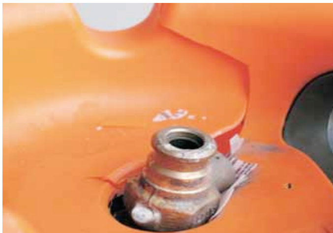
Figure 4 Domage structurel (niveau 3) – irréparable
